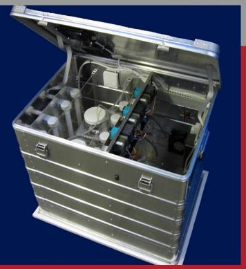
The algae cultivated in the AFD are planktonic and unicellular. Nutrients, trace elements,  $CO_2$  and light are the key elements necessary for algal growth. In the AFD algae (*e.g. Chlorella* sp.) are cultivated to a high density by a chemostat lag-phase approach. Nutrients are continuously added, the algal suspension is offered as food for the bivalves in the Mosselmonitor. With this continuous supply of food mussels keep their shells open (even in drinking water).
